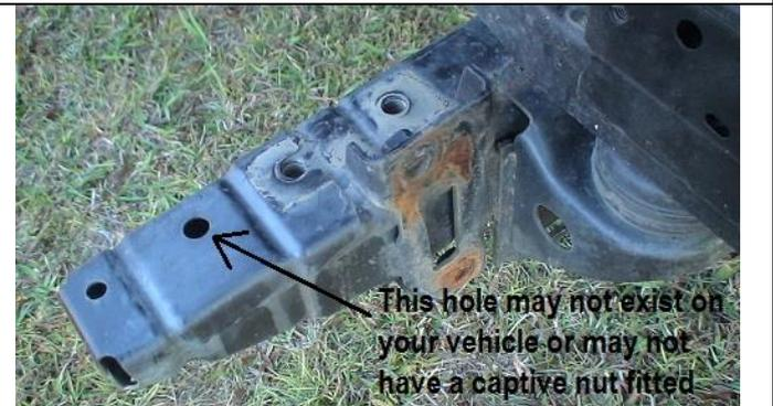
Take the cradle and winch assembly and sit it on the chassis rails. Secure the cradle at the front two mounting points with the bolts, spring washers and flat washers supplied. Refer image.
