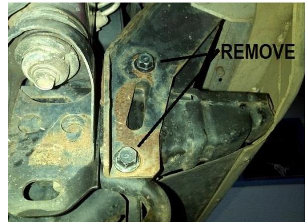
Remove the bolts securing the bullbar to the top of the chassis rails.
