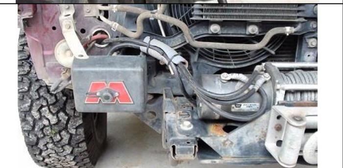
**Note:** Remove the spacer between the bullbar mounting bracket and the chassis rail in the location shown. This gap is taken up by the thickness of the winch cradle.
