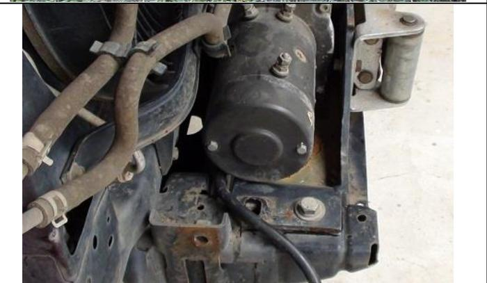
At This point you need to determine the location in which to mount the control box for the winch. There is no set location however some suggestions are behind the bulbar wing (as shown), top pan of bulbar or under bonnet. The location will depend totally on yourself and your requirements.
