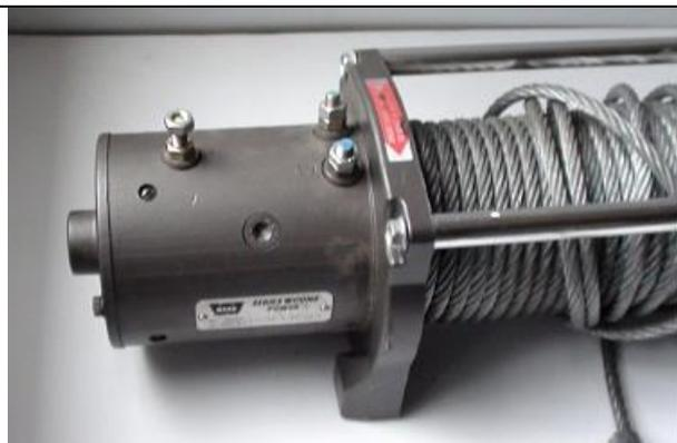
Using the four bolts, flat washers and spring washers supplied with the winch, secure the winch to the cradle
